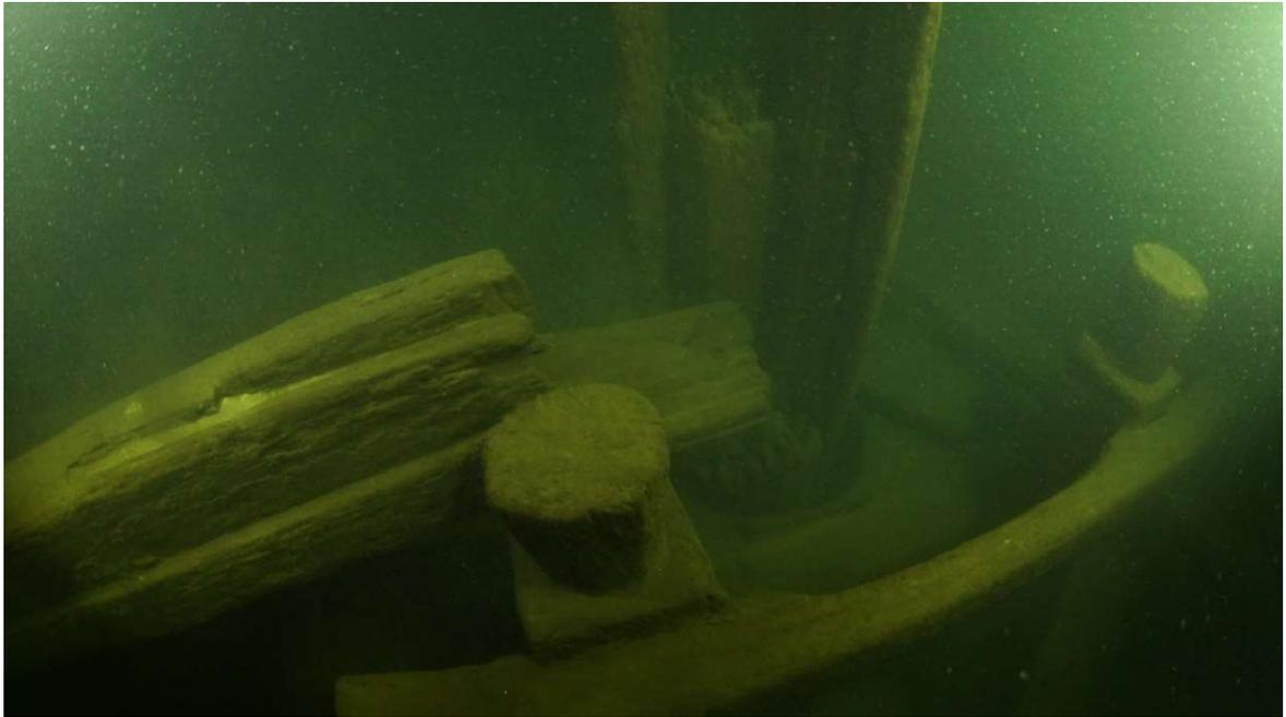
Fig. 39. Jeerbitts behind the main mast. Video frame capture: Kari Hyttinen.
