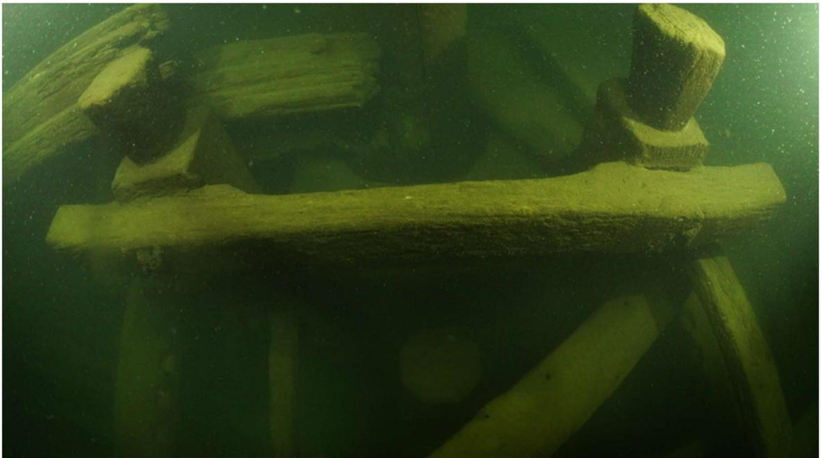
Fig. 40. Jeerbitts behind the main mast. Video frame capture: Kari Hyttinen.
