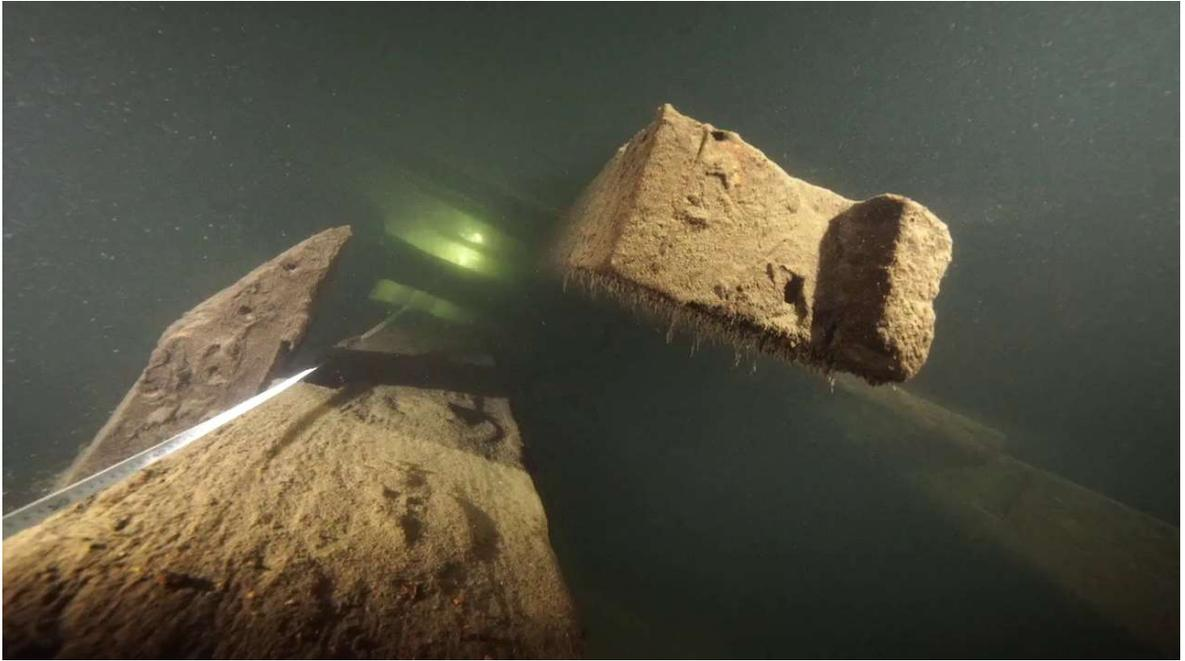
Fig. 32. Measuring of the wing transom. Video frame capture: Kari Hyttinen.
