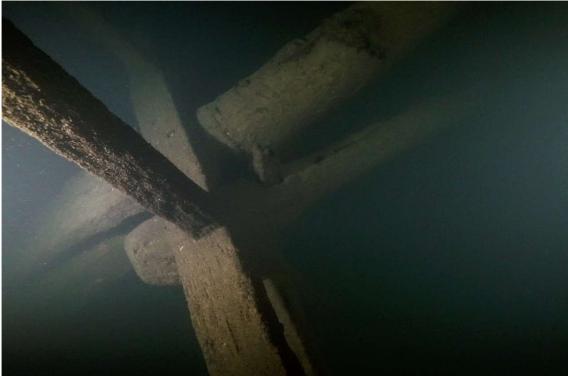
Fig. 10. Mizzen crosstrees and topmast. The chock that prevents the topmast to fall down thru the crosstrees, is also visible in the middle of the image. Frame capture from video by Immi Wallin.
