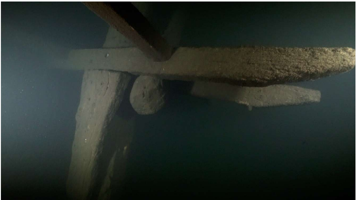
Fig. 9. Mizzen crosstrees and lower end of topmast. Frame capture from video by Immi Wallin.
