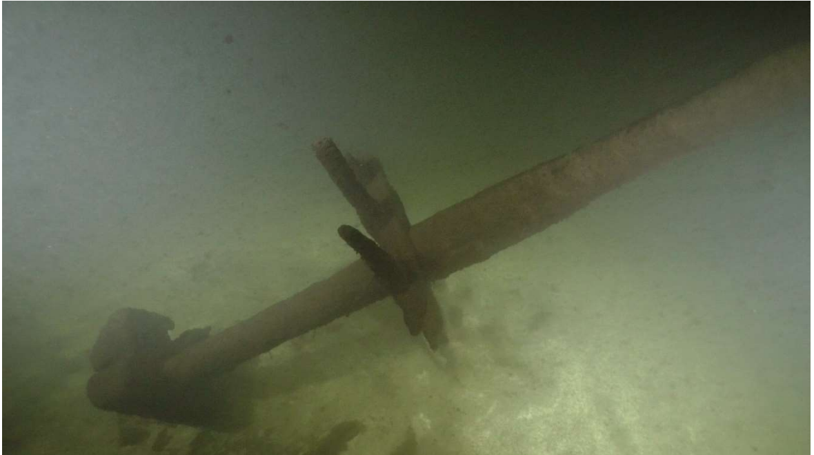
Fig. 6. Mizzen top mast with crosstrees and mastcap. Frame capture from video by Immi Wallin.
