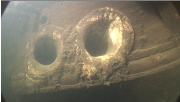
Picture 55. Hawse holes on the starboard side. Photo by P. Raasakka & J. Kaasinen.
