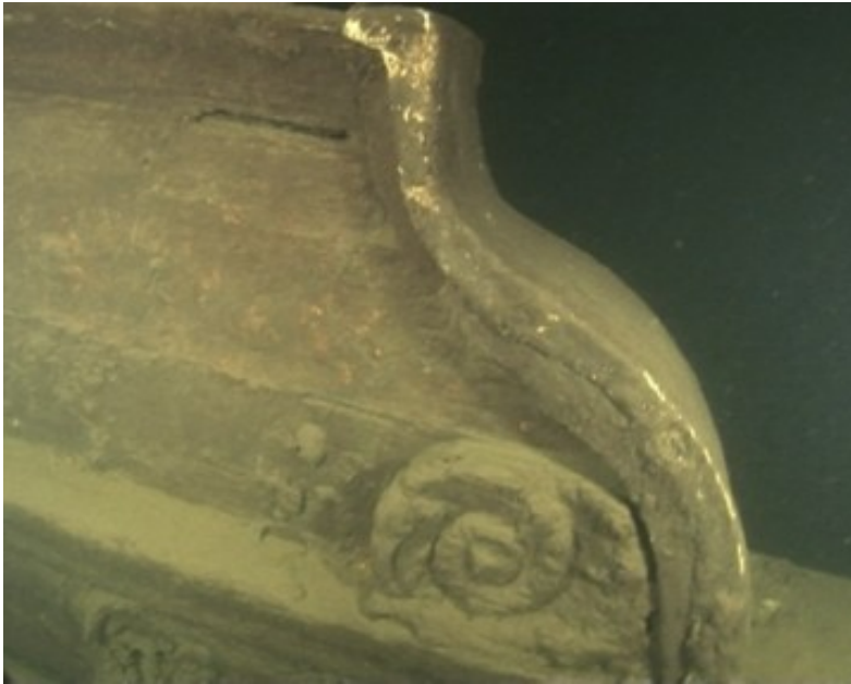
Picture 35. The gunwale break on the starboard side near the fore edge of the poop deck (viewed from outside of the ship). Photo by P. Raasakka & J. Kaasinen.
