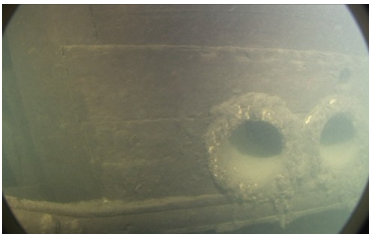
Picture 56. Hawse holes on the port side. Photo by P. Raasakka & J. Kaasinen.
