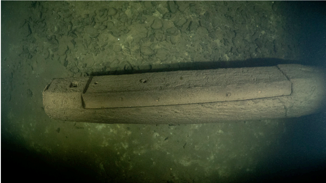
Figure 81: (E) The end of a boom. Whether this is part of fore mast, or something else, is not known. The missing bowsprit had a very similar cut cutout in the end. However it is unlikely that this object could be the bowsprit as it lacks some of the features of the bowsprit, and because the other end is below several objects in front of the stem post. It could be an extension of the bowsprit, i.e. a jibboom. Photo 30th August 2020.
