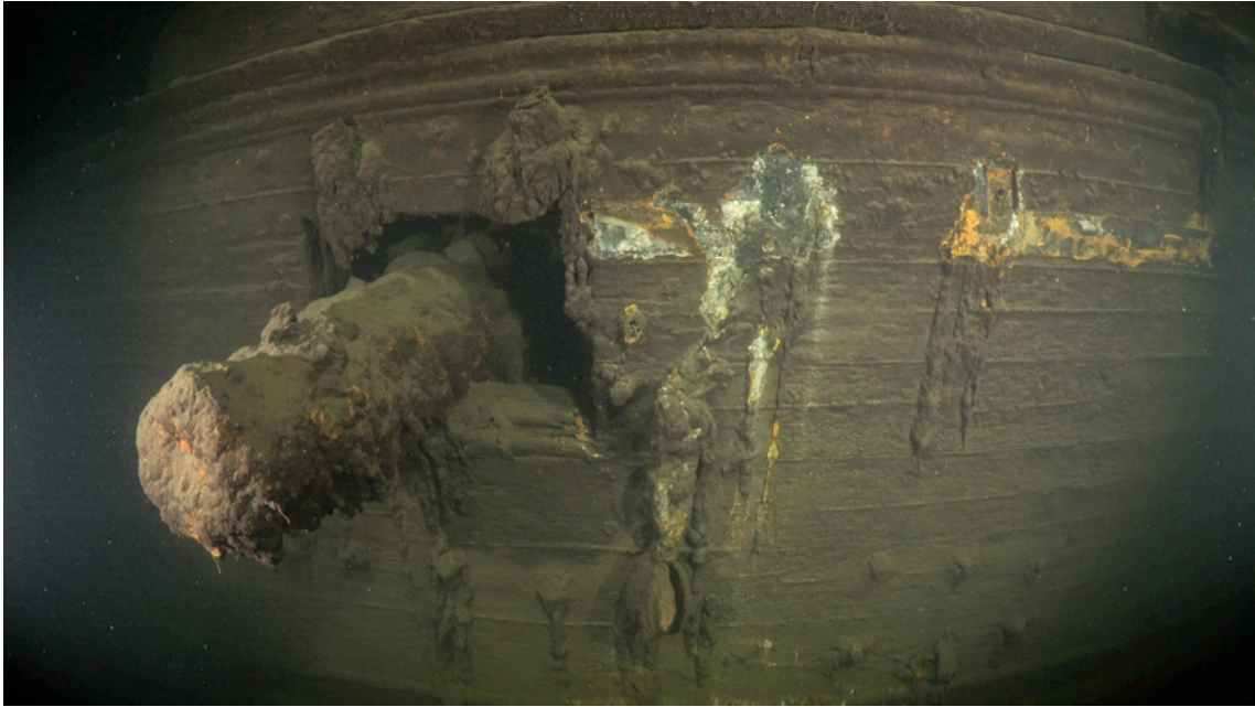
Figure 56: The port side gun closest to the stern. The marks on the right next to the upper edge of the gunport mark the location where the mizzen channel has been, and a deadeye is still hanging from it on a remains of a rope. The channel has fallen down and is probably on the bottom below. The channel has fallen before the discovery of the wreck. Videocaption 23rd July 2019.
