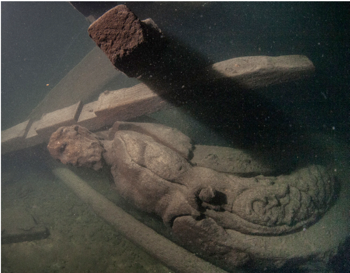
Figure 74: The figure head still in the condition it was found (11th August 2007, photo Jouni Polkko). The beam pointing towards the camera is one of the trestletrees of the fore mast. In front of the figure head is a loose crosstree from the fore mast. The fore mast is behind the head figure.
