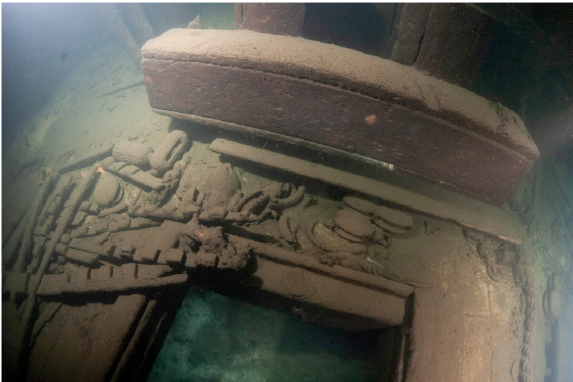
Figure 29: The crossbeam abaft the riding bitts. Loose items on the deck; blocks, remains of ropes and remains of a wooden grating. Photo 11th September 2011.
