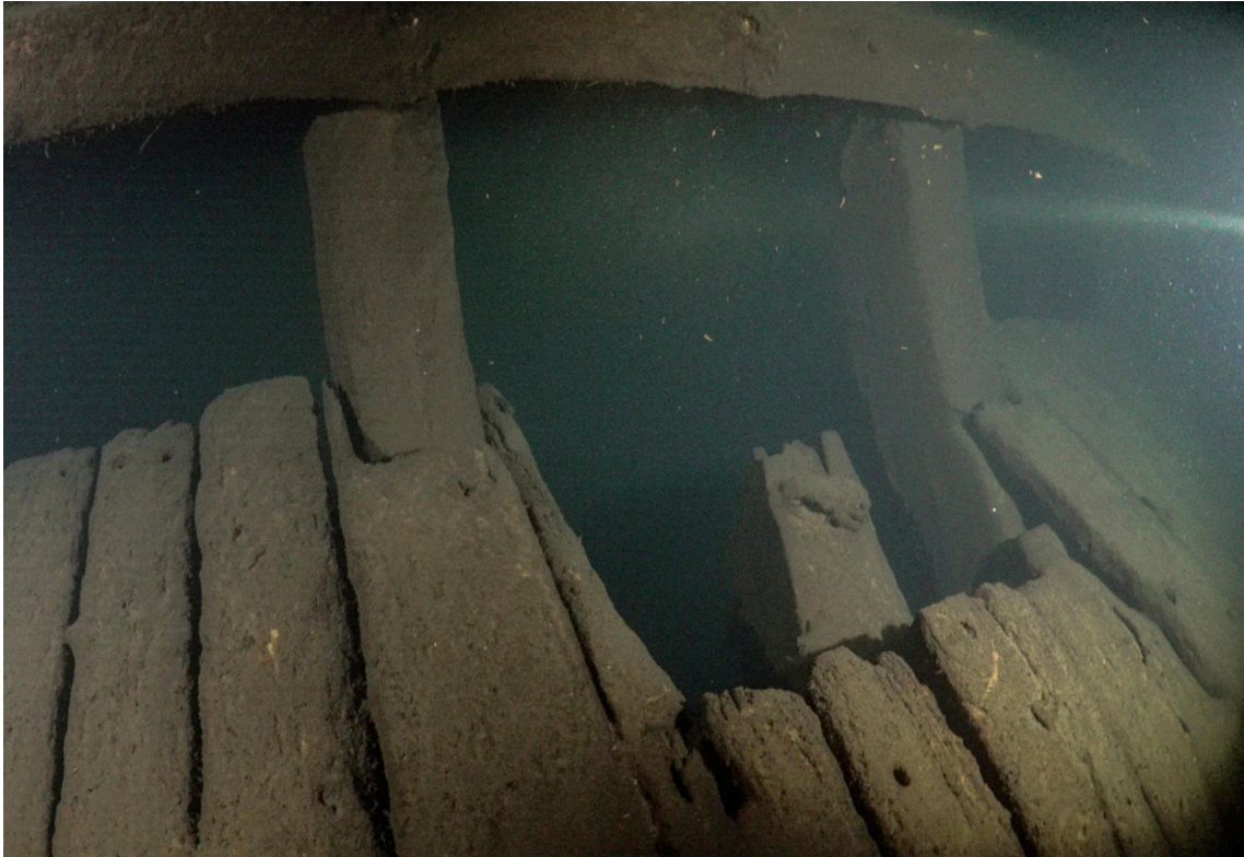
Figure 53: Inside the stern cabin (view towards transom). The tiller is still visible inside the deck plank cutout. The helm port has been here.
