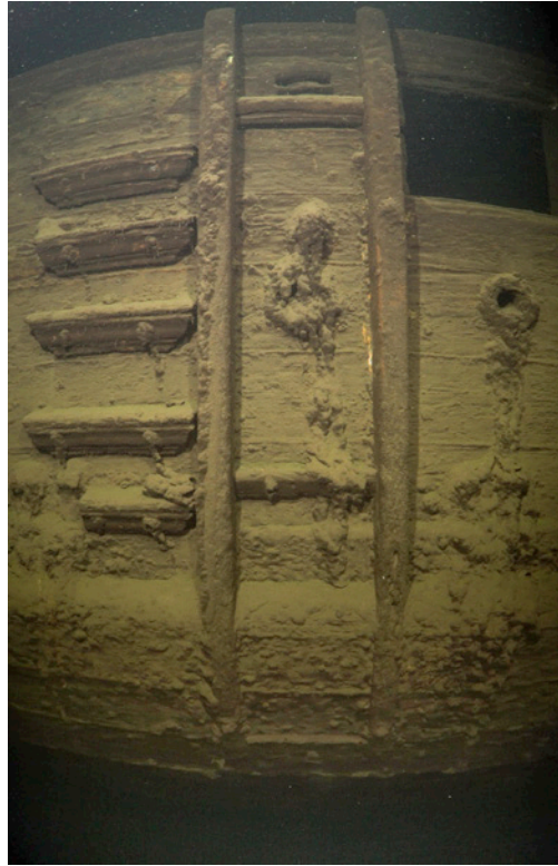
Figure 66: Details on the starboard side of the hull, a little bit forward from the main mast. Entry steps can be seen on the left. In the middle, there are two fenders. Between these fenders, the gunwale has two embedded sheaves for the fore sheet. Drain holes can be seen below the gunport there and between the fenders (for letting water out from the deck). The main wale is just under the entry steps. Above the main wale, there are two small lids with two corroded hinges. These features look like sweep ports. Videocapture 12th August 2020
