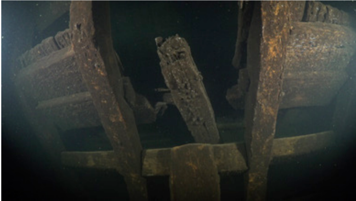
Figure 58: A view upwards below wing transom, towards the tiller and and the tiller port. The tiller is in the middle and the stern post below. Videocapture 8th August 2020.
