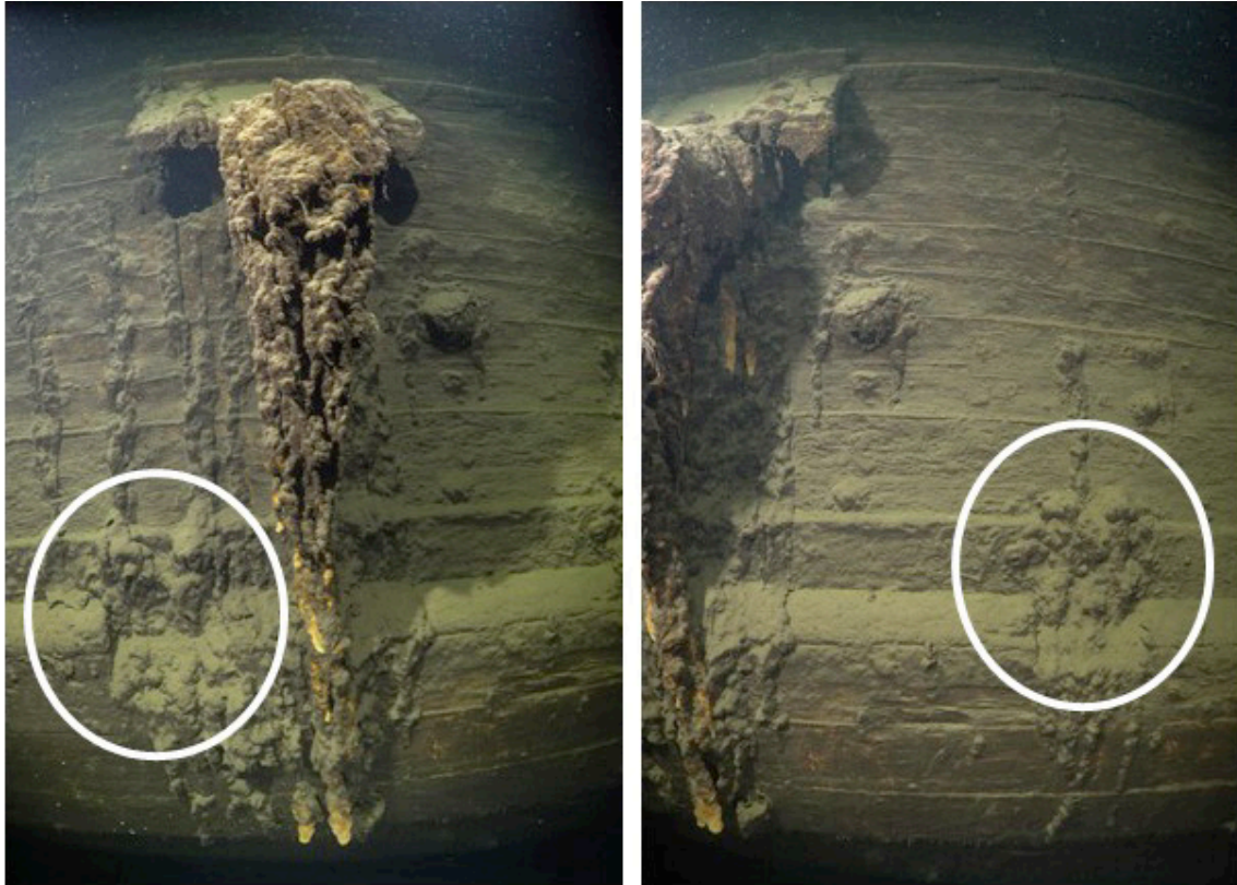
Figure 68: Presumed sweep ports closest to the stern on the starboard side. There are cutouts in the main wale, which could be for allowing the movement of the oars and the sweep port lid to open. It is also possible, that shorter oars were used in the stern, where the ship is narrower, requiring a steeper angle downwards for rowing. Videocapture 12th August 2020.
