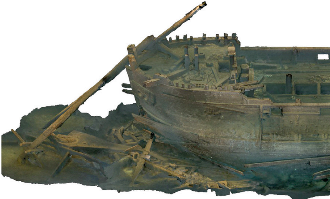
Figure 7: Orthometric view capture from the 3D photogrammetric model shows the bow and forecastle area.
