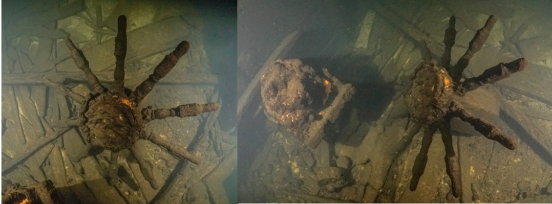
Figure 33 (left): The wheel of the ship. The root of the mizzen mast is visible on the right image. The loose planks behind the wheel are possibly the remains of the stern cabin wall. Videocapture 6th August 2019.
