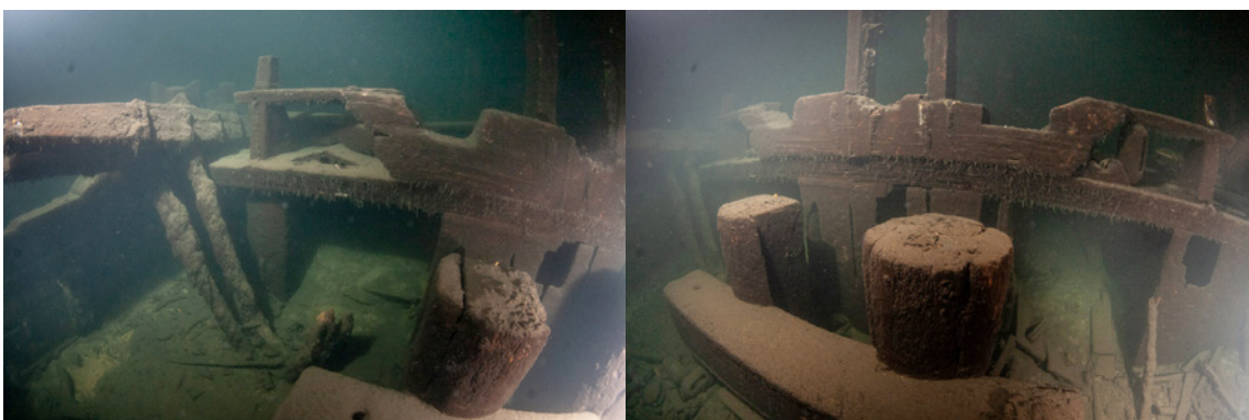
Figure 13: The image on left shows the aft end of the forecastle and a break on the port side. There are two spare anchors on the left. The image on right shows the forecastle aft and a break in the starboard side. The crossbeam for supporting rigging spare parts like topmasts is visible. There is an open access below the forecastle in both sides. Photo 11th September 2011.
