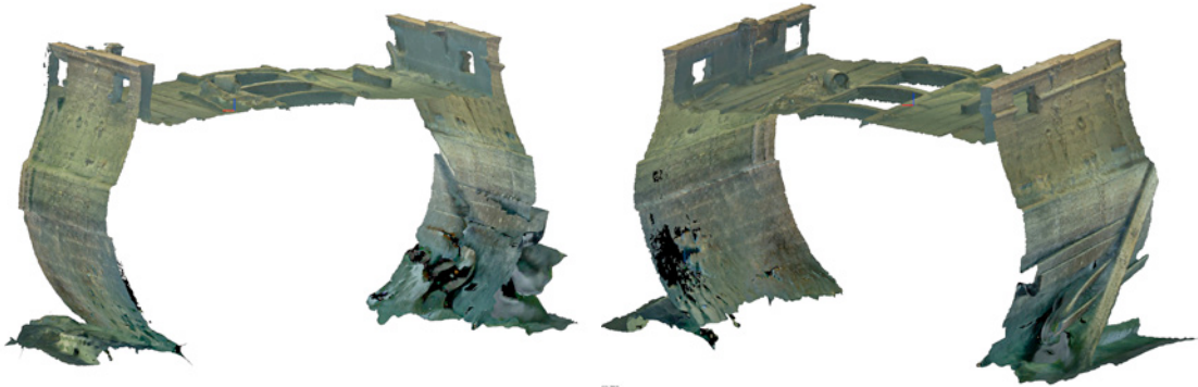
Figure 61: Orthometric 3D cross-sections close to the widest point of the hull. The starboard side is shown on the left, and the port side on the right. The hull is widest at the main wale. The main wale consists of three planks. There is a narrow strake above the main wale. The hull is practically intact around the mid-ship area on the starboard side. on the port side, there are some loose planks below the main wale.
