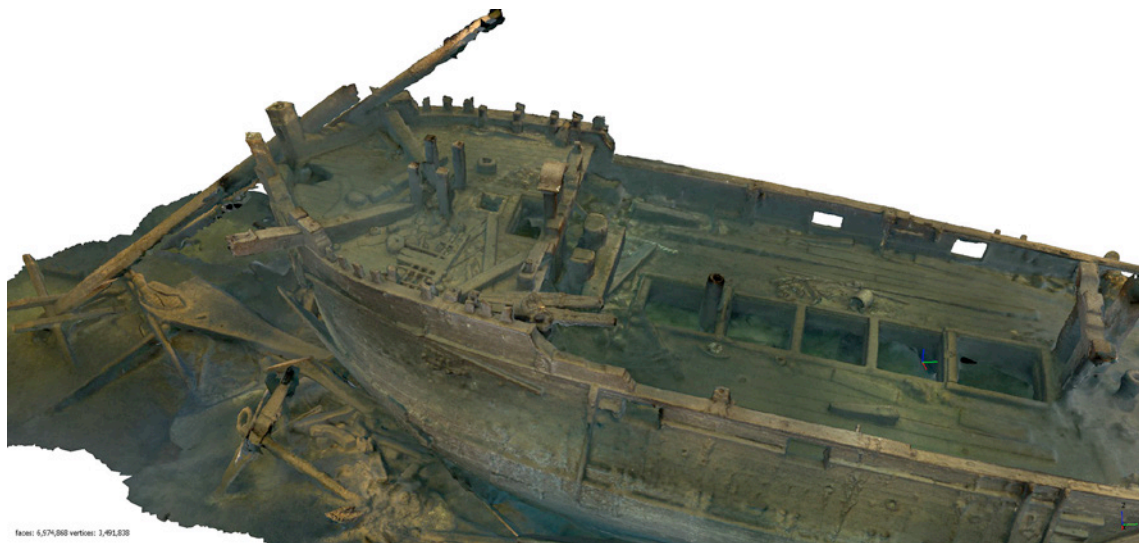
Figure 15: This birds-eye-view shows the fore-castle, break and part of the gun deck up to the main mast (which can be seen far right). In front of the main mast there is another cross beam supported by two bitts. This crossbeam has two non-symmetric grooves and has supported the other ends of the spare topmasts laying horizontally. Stocks of two spare anchors on the gun deck are visible in port side, the stocks are just above the fore-castle.
