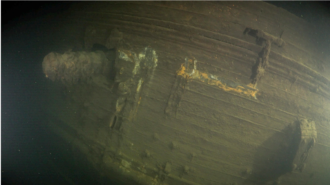
Figure 70: The first gun from the stern on the port side can be seen on the left. There are clear marks where the mizzen channel has been (on the level of the gunports' upper edge). It looks like the mizzen channel has had two separate channel plates. The small dark dots are probable attachment point for chain plates. There is a fixed rectangular block with shieves on the right corner. Videocapture 23rd July 2019.
