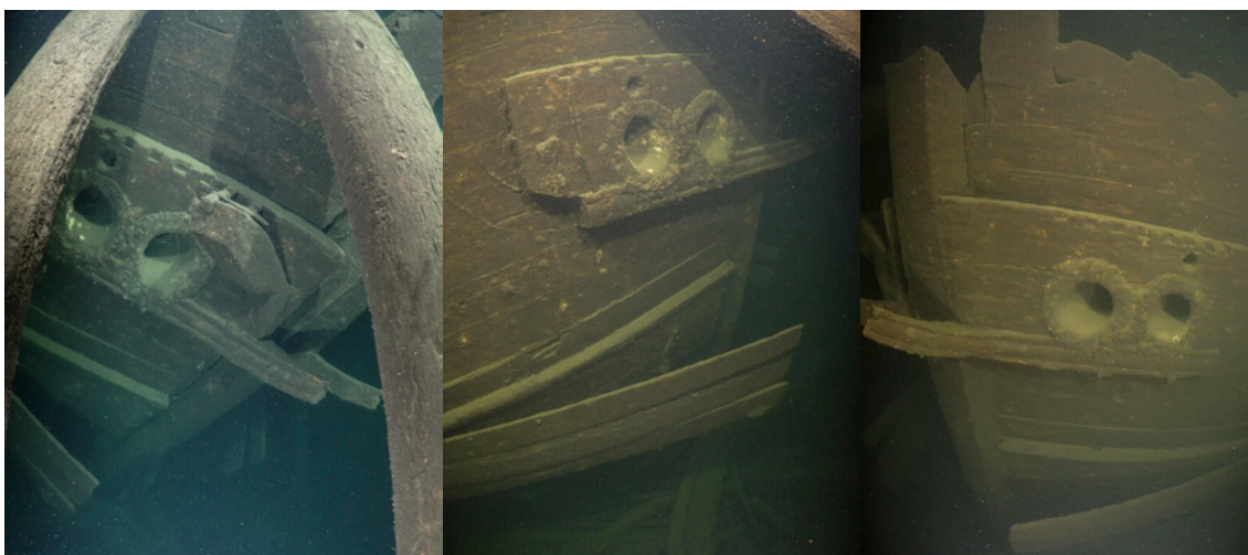
Figure 64 (left and center): Hawse linings and hawse holes on the starboard side of the bow. Hair brackets below hawse holes and lining are still partly intact. Main wale planks have become loose close the bow and have detached from stem post. Videocaptures 12th August 2020.
