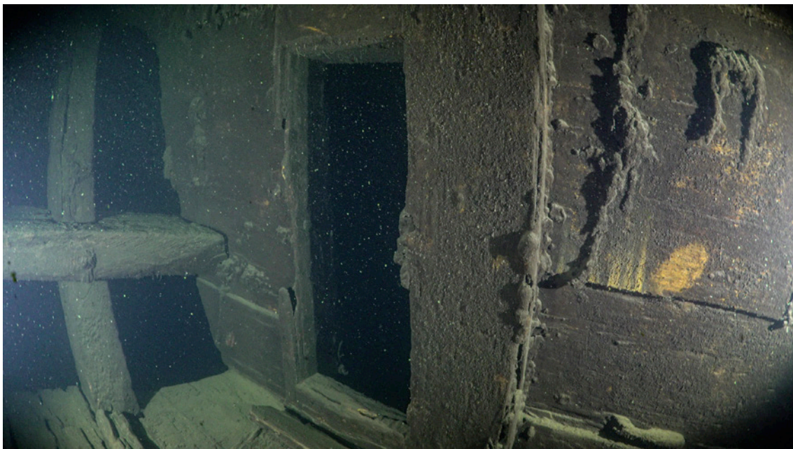
Figure 52: A view inside stern cabin. The access hatchway into the port side quarter gallery can be seen in the middle. Stern lights on the left. Videocapture 25th August 2019.
