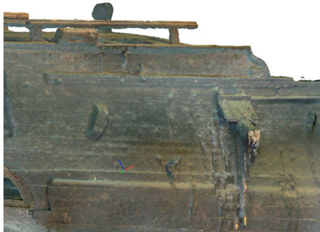
Figure 43: This on gun the starboard side closest the stern has almost slid out through the gunport. The gun points downwards in apporox. 35 degree angle. The lid on this gunport opens from above the gunport. This same gun is shown from the deckside in the figure 45. Note the ornament carving in the gunwale break. Three planks of the main wale are visible. 3D photogrammetric model.
